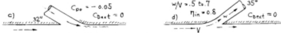
Figure 28. Pressure coefficients (and estimated drag coefficients) of several marine-type condenser-water outlets (21) and of one inlet opening.
